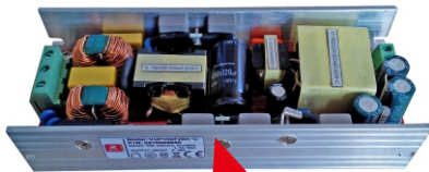
Item number: M1000954A VUP150F28A344 IN:100-240VAC 50/60Hz OUT:28VDC 5.36A 150W Power supplier
